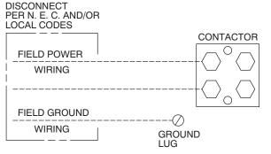
Fig. 8 - Line Connections
